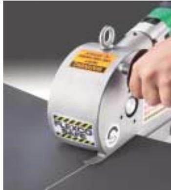
The Electric Belt Cutter is available in two sizes and specifically designed to allow the end user to cut belts quickly and safely resulting in less conveyor downtime, and overall increased productivity. The EBC1 Electric Belt Cutter is capable of cutting a rubber belt up to 1" (25 mm) and up to a maximum 360 P.I.W. (630 N/m) on PVC belts while the EBC2 cuts rubber belts up to 2" (50 mm) and up to a maximum 1140 P.I.W. (2000 N/m) on PVC belts.
