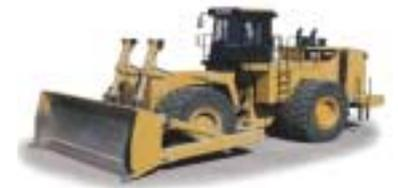
The 854K replaces the 854G and retains the best features, including the impeller clutch torque converter for superior operator control and optimum power to the ground, lockup clutch for direct drive efficiency, and STIC™ control system for reduced steering and transmission control effort.
